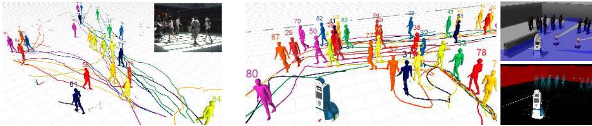
Fig. 3. Example groundtruth tracks of the datasets used in our experiments, and originating laser endpoints (in grey). Left: Freiburg Main Station dataset, recorded with a stationary LMS 291 laser scanner. The camera image is only for visualization purposes. Right: Synthetic dataset generated by combining the pedestrian simulator PedSim with Gazebo to simulate 2D laser range data via raycasting (small pictures). Our simulation is modelled after a highly crowded, real airport scenario where people disembark from an airplane and enter the airport terminal. The simulated robot is driving through the 30\text{m} \times 30\text{m} scene for exploration and equipped with two laser scanners at 70 cm height.
