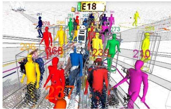
Fig. 1. Typical example of a crowded, dynamic situation in an airport terminal with frequent occlusions where we want to robustly and efficiently track persons from a first-person perspective with our mobile service robot platform, which can (barely) be seen in the middle of the picture.
