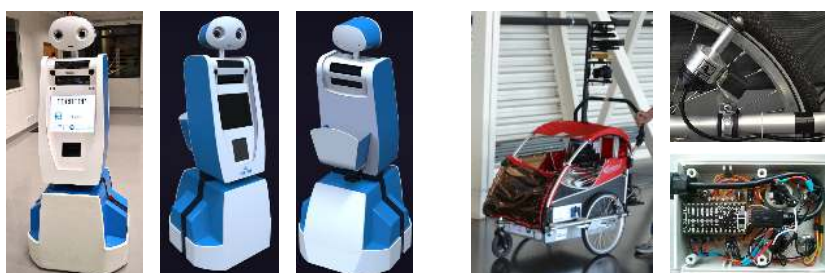
Fig. 2. Left: Picture and renderings of the SPENCER robot platform. Right: The custom-built mobile data capture platform, including a custom odometry solution using quadrature encoders in dynamo housings on both main wheels, connected to a microcontroller (bottom right picture). Both platforms contain numerous ROS-based software components distributed over multiple computers.
