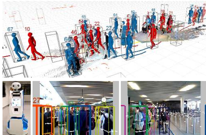
Fig. 1. Typical example of a crowded, highly dynamic situation in an airport terminal where we want to robustly and efficiently track persons with our service robot platform depicted on the bottom left.
