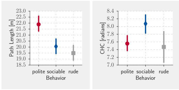
Fig. 5. Navigation results in the lobby scenario using polite, sociable and rude behaviors showing the two objective metrics path length and path smoothness in terms of numbers of heading changes along the path. Intervals show 95% confidence from 15 different runs.
