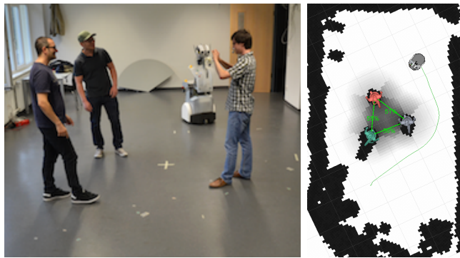
Fig. 1. Socially normative behavior example. Three persons are engaged into a photography activity and the robot should not drive through the group even though there is enough space and the path would be shorter and smoother. The corresponding costmap from the learned model is shown on the right, with darker cells having higher costs. The strength of the social relations between individuals are indicated in percent.
