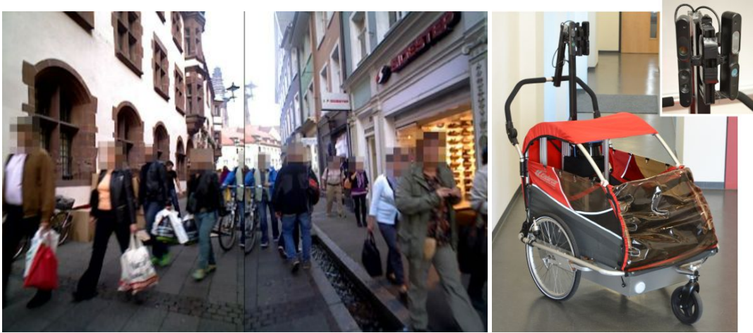
Figure 5: Left: the Rathausgasse (Freiburg) dataset, captured in a crowded pedestrian zone in multiple runs over a distance of 300 meters. It contains color and depth camera images, as well as distance measurements from a 2D laser range finder. Right: the mobile data capture platform that was built at the beginning of the SPENCER project to capture scenarios like this. It is equipped with a SICK LMS-500 laser range finder, custom-built wheel encoders for odometry, and two vertically mounted Asus Xtion Pro Live RGB-D sensors. The orientation of these sensors will be changed in the future to reflect the actual setup on the SPENCER robot platform.
